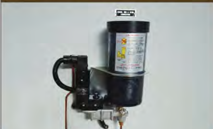
Automatic Grease Lubrication System
